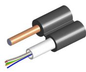
Fiber drop cable, LightScope ZWP® Self-Supporting Non-Armored Figure-8, Singlemode G.652.D and G.657.A1, 2 fiber Arid Core construction with 0.064 in solid messenger, Gel-filled, central loose tube, Feet jacket marking, Black jacket color
