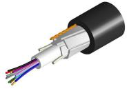
Fiber indoor/outdoor drop cable, LightScope ZWP® All-Dielectric, Singlemode G.652.D and G.657.A1, 12 fiber Arid Core construction, Gelfilled, low smoke zero halogen (LSZH), central loose tube, Meters jacket marking, Black jacket color, Dca flame rating
