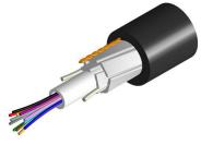
Fiber indoor/outdoor drop cable, LightScope ZWP® All-Dielectric, Singlemode G.652.D and G.657.A1, 12 fiber Arid Core construction, Gelfilled, low smoke zero halogen (LSZH), central loose tube, Meters jacket marking, Black jacket color, Dca flame rating
