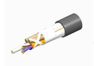
Fiber indoor/outdoor cable, LightScope ZWP®, Single Jacket All-Dielectric, Plenum Rated, Singlemode G.652.D and G.657.A1, 72 fiber, Gel-Free, Stranded Loose Tube, PVDF jacket, Feet jacket marking, Black jacket color
