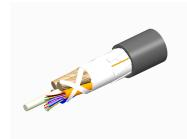
Fiber indoor/outdoor cable, LightScope ZWP®, Single Jacket All-Dielectric, Plenum Rated, Gel-Free, Singlemode G.652.D and G.657.Al, 24 fiber, Stranded Loose Tube, PVDF jacket, Feet jacket marking, Black jacket color
