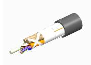
Fiber indoor/outdoor cable, LightScope ZWP®, Single Jacket All-Dielectric, Plenum Rated, Singlemode G.652.D and G.657.A1, 6 fiber, Gel-Free, Stranded Loose Tube, PVDF jacket, Meters jacket marking, Black jacket color
