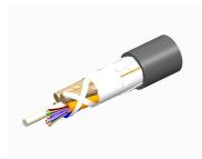
Fiber indoor/outdoor cable, LightScope ZWP®, Single Jacket All-Dielectric, Plenum Rated, Singlemode G.652.D and G.657.Al, 6 fiber, Gel-Free, Stranded Loose Tube, PVDF jacket, Meters jacket marking, Black jacket color
