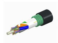
Fiber OSP cable, LightScope ZWP® Single Jacket/Single Armor, 84 fiber, Gel-Free, Stranded Loose Tube, Singlemode G.652.D and G.657.A1, Meters jacket marking, Black jacket color
