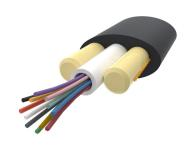
Fiber outdoor drop cable, LightScope ZWP® Self-Supporting All-Dielectric, Singlemode G.652.D and G.657.Al, 6 fiber Arid Core construction, Gel-filled, central loose tube, Meter jacket marking, Black jacket color
