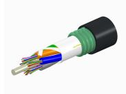
Fiber OSP cable, LightScope ZWP® Single Jacket/Single Armor, 84 fiber, Gel-Free, Stranded Loose Tube, Singlemode G.652.D and G.657.A1, Feet jacket marking, Black jacket color
