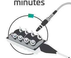
Use of pre-terminated connectors eliminates splicing, thus reducing the total time of connecting a customer to the fiber network
