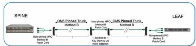
Figure 6: MPO-8 – QSFP breakout applications – 4 duplex ports
