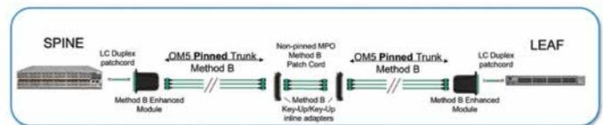
Figure 7: MPO-8 – Parallel cabling
