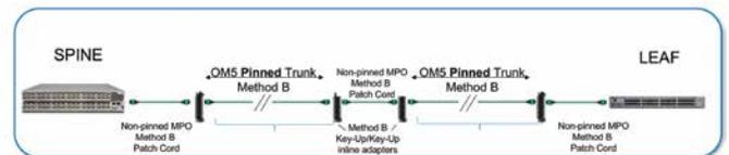
Figure 15: 100G and 120G parallel support with MPO-24
