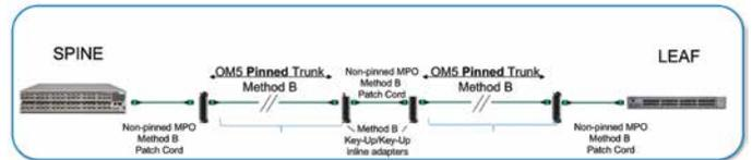
Figure 5: MPO-8 – Parallel cabling
