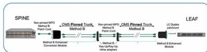
Figure 11: Three port QSFP module supported with two MPO-12 trunks
