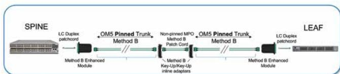
Figure 9: MPO-12 group of 2 trunks for 12 LC ports
