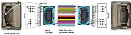
Figure 4: MPO-8 – QSFP applications with method B polarity management
