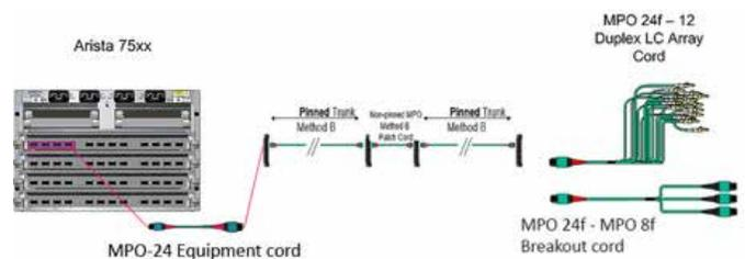
Figure 16: 120G parallel support with MPO-24
