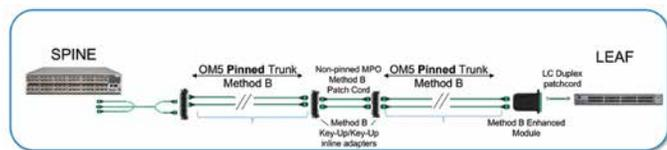
Figure 10: MPO-12 modules and fan-out assembly example
