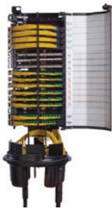
In response to aesthetic and concealment challenges faced by municipalities deploying urban FTTH, CommScope has designed the sealed **FDH 4000**. This is an underground preterminated fiber flexibility point system for the point-to-point and splitter/WDM-based connection between feeder and distribution point.
