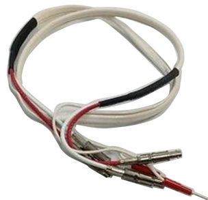
DS3 Cross-connect Patch Cord, Coax, dual, BNC to LCC, white, 50 ft
