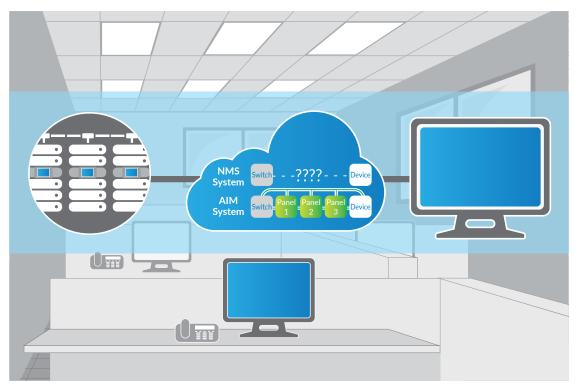
The AIM system can provide detailed end-to-end physical connectivity information to a network management system
