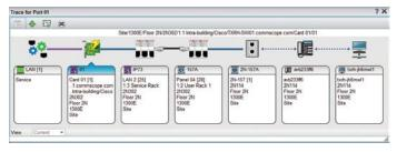
A detailed end-to-end trace from CommScope's imVision® AIM solution
