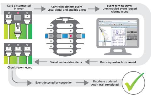
Figure 1: Automated incident management with an AIM system
