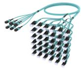
Ultra Low Loss ULL LazrSPEED® 550 MPO(Pinned) to LC/UPC Uniboot Ruggedized fanout Cable, 72-Fiber, Plenum, 12 fiber PmP 2.0 mm Dca
