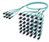
Ultra Low Loss ULL LazrSPEED® 550 MPO(Unpinned) to LC/UPC Uniboot Ruggedized fanout Cable, 72-Fiber, LSZH, 12 fiber PmP 2.0 mm /B2ca
