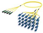
Ultra Low Loss ULL TeraSPEED® MPO(Pinned) to LC/UPC Uniboot Ruggedized fanout Cable, 48-Fiber, LSZH, 12 fiber PmP 2.0 mm /B2ca
