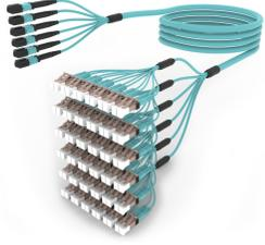
OM4 MPO (Unpinned) to LC/UPC, InstaPATCH® 360 Ruggedized Fanout Cable, 72-Fiber, Plenum
