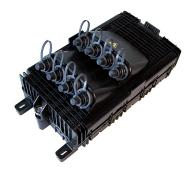
Mini-OTE 300-Series, Optical Terminal Enclosure, 8-port full-size connector, 1x4 tap, 17dB, with thru port, black, with grounding, external mounting
