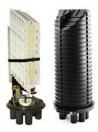
FOSC® 400 D5 Fiber Optic Splice Closure, Heat Shrink Cable sealing, one pre-installed 72-splice tray, cable blocking, with test valve
