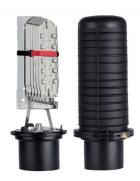
FOSC® 450 B6 Fiber Optic Splice Closure, Gel Cable sealing, one pre-installed 24-splice tray, 6 cable attach., three ground feedthrough lugs, with test valve
