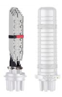
FOSC® 400 B4 Fire Retardant Fiber Optic Splice Closure, Heat Shrink Cable sealing, no pre-installed trays, ground feedthrough lugs, with test valve
