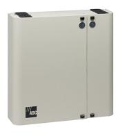
FL1000 Fiber Wall Box, 2-door, singlemode FC/UPC, 24-ports, with pigtails and splice tray, 2 cable clamps, 2 compression fittings, 2 grounding kits, 2 strength member tie-offs, 2 key locks
