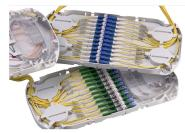
FIST GPST Fiber Patch/Splice Tray, 12 ports, FC/APC, singlemode, preterminated with pigtails, SMOUV splice chip, 19 in, gray, right patch cord routing
