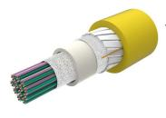
Fiber indoor cable, All-Dielectric, LSZH/Riser-Rated, Gel-Free, Central Tube Rollable Ribbon, 192 fiber, Singlemode G.657.A2/B2, Feet jacket marking, Yellow jacket color, Cca flame rating
