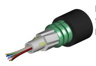
Fiber drop cable, TeraSPEED® Single Jacket Single Armor Arid-Core, 4-fiber, Singlemode G.652.D and G.657.A1, gel-filled, Feet jacket marking, Black jacket color
