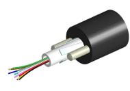
Fiber drop cable, TeraSPEED® Single Jacket All-Dielectric Arid Core, 12-fiber, Singlemode G.652.D and G.657.Al, Gel-filled, Feet jacket marking, Black jacket color
