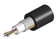
Fiber Indoor/Outdoor Drop Cable, TeraSPEED®, Low Smoke Zero Halogen Single Jacket All-Dielectric Arid-Core, 6 fiber, Gel-filled, Singlemode G.652.D and G.657.A1, Feet jacket marking, Black jacket color, Dca flame rating
