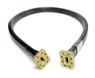
FlexTwist® Flexible Twist for WR112, 7.125–8.5 GHz, with interface types CPR112G and UBR84, 1200 mm
