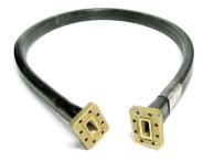
FlexTwist® Flexible Twist for WR75, 10.0–15.0 GHz, with interface types PBR120 and PBR120, 300 mm
