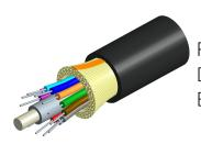
Fiber indoor/outdoor cable, LazrSPEED® Zero Halogen Riser Distribution, 2 fiber single-unit, Multimode OM3, Feet jacket marking, Black jacket color, Dca flame rating
